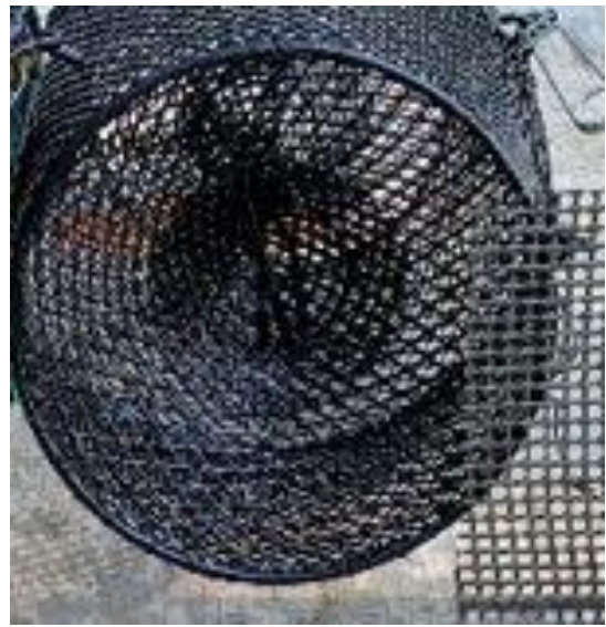
Step 4: Press the mesh trap. Secure it in the metal cone with a medium cable tie.
