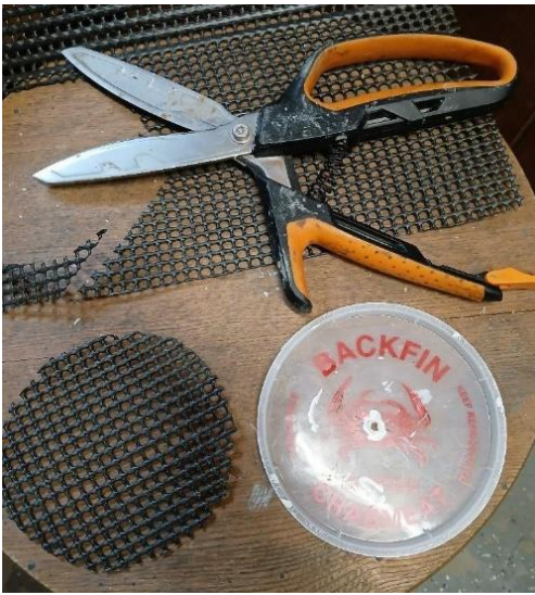
Step 1: start by cutting two circular pieces from a scrap of small mesh spat bag.
